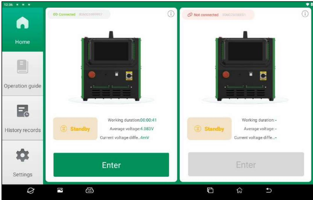
If the detection tablet hasn't been connected to the CE39 before, the app will open the device search page upon startup. Follow the on-page instructions to connect power to the CE39, turn on its DC and AC switches, and wait for the green light on top of the device to light up.
