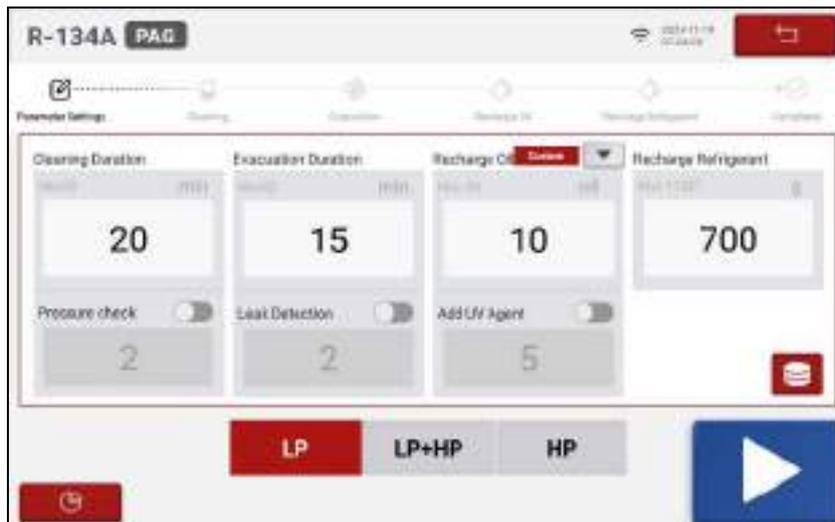
Click the numerical display area of each parameter, and then use the keypad to modify the parameter.
