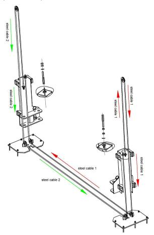
Step7: Mount the power unit onto the power side post.
