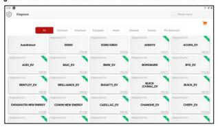
2) Click on the corresponding brand of the vehicle to be inspected, here we take Demo (Version 15.54) as an example to demonstrate how to diagnose a vehicle.
