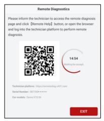
Notify the service technician to assist in remote diagnosis. You can take a picture of the dialog box shown above and share it with the technician, who can scan the QR code and log in to the technician platform for remote diagnosis, or carry out remote diagnosis based on the serial number of the inspection connector, the owner's cell phone number or the license plate number provided by the user.
