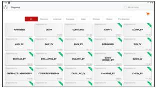
Some models may not be able to identify the vehicle information through the AutoDetect function, then the following dialog box will pop up for the user to scan or manually enter the vehicle VIN code.
