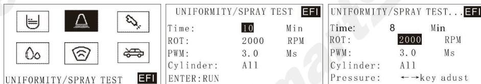
Uniformity test is to find out the difference of the injectors injecting at the same working condition. This test can indicate the comprehensive influences on the injector caused by electrical nature, bore variation and clogging. Spray ability test is to inspect the spraying performance by observing the injectors.
