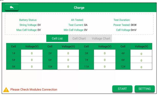
The current battery status, the test current, the test duration, the current voltage of the battery pack and the cell information can be viewed on the test interface. The configuration can be modified during the test.
