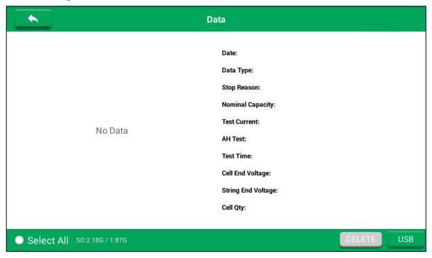
Insert a U-disk into the USB port on the panel, select the data to be saved, and tap USB button to transfer the corresponding discharge data and charge data to the U-disk.
