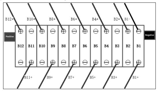
According to the wire label on the equalization subharness, B1 - is connected to the negative electrode of No. 1 single cell (B1), B1 + is connected to the positive electrode of No. 1 single cell (B1), B2 + is connected to the positive electrode of No. 2 single cell (B2), and connected in sequence.
