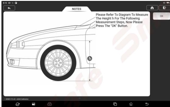
Follow the on-screen instructions to measure the height H (from the tire contact surface to the wheel housing edge) of each wheel respectively, and input the actual measured values.
