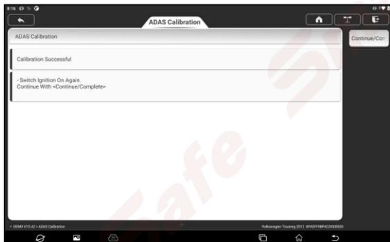
Switch the ignition on again, tap **Continue/Complete** to code the driver assistance systems front camera data into the vehicle's ECU.
