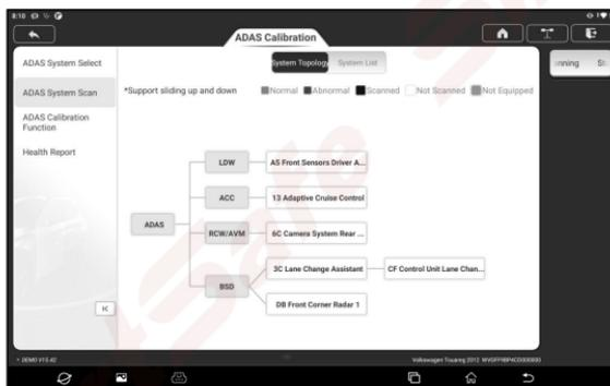
The ADAS systems can be displayed in form of topology or list. Tap **Start Scanning** to start reading DTCs. After scanning is complete, tap the system displayed in red to view the existing DTCs, or tap the system functioning normally to perform other diagnostic functions.
