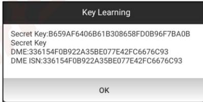
11. Place a new key close to vehicle coil, tap **OK**, and wait for key generation.
