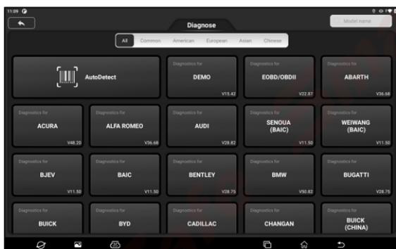
2. Click the vehicle brand to be tested to enter the model version information interface. Here we take Demo (Version 15.42) as an example to demonstrate how to diagnose a vehicle.
