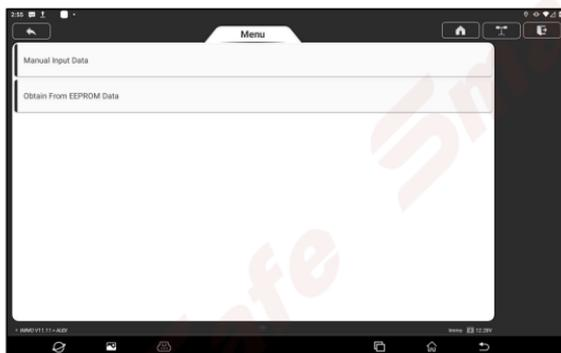
2) Tap **Edit2**, if you have obtained the relevant data of the original vehicle gearbox from other equipment, select **Manual Input Data** and enter the 16-byte CS code of the original vehicle gearbox.
