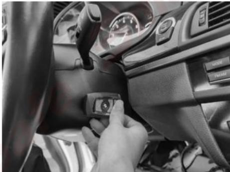
12. After the dealer key is successfully generated, please try to start the vehicle. Now the key matching is finished and the new key is ready for use.
